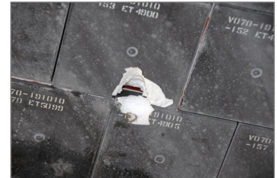
Damaged carbon-carbon panel
